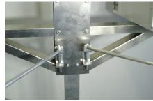
Step 12: Check all bolts making sure they are securely tightened before raising your housing. Your Multipurpose is now ready to be raised! When you reach the top of the pole and are against the stop, DO NOT over tighten or damage may occur.
