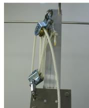
**Step7**: Attach the rope winder to the pole at your desired height using two 1/4 x 2-3/4 bolt with 1/4 flange nuts. The rope winder needs to be oriented so that when the rope is wound, the rope extends straight down from the eyebolt. The rope can not be twisted around the pole or excessive wear will occur.
