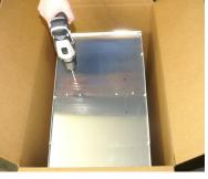
**Method A; Step 5:** Mount the Martin House to the mounting plate using 3/4" bolts with flange nuts.
