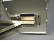
**Method B; Step 2:** Drill 1/4" hole at the marked location. Repeat this process for the remaining martin house.
