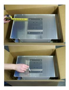
**Method A; Step 3:** Drill 1/4" holes at the marked locations. Repeat this process for the remaining martin house.
