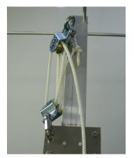
Step 7: Attach the rope winder to the pole at your desired height using
