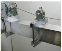
**Step 10:** Thread the winch handle onto the winch. Slide the spring onto the winch beside the handle. Secure the spring with the 3/4" wide nut.
