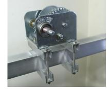
**Step 9:** Attach the cable guide pulley approximately 10" above the winch using one aluminum u-channel and  $1/4 \ge 4-1/2$ " bolts and flange nuts.
