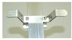
**STEP 8**: Attach the rope winder to the pole at your desired height using two 1/4 x 2-3/4 bolt with 1/4 flange nuts. The rope winder needs to be oriented so that when the rope is wound, the rope extends straight down from the house. The rope can not be twisted around the pole or excessive wear will occur.
